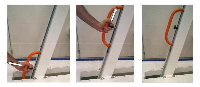
The heights are shown on the shaft next to the bracket for the height adjustment.
